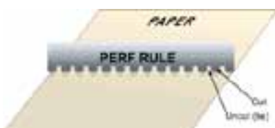
PERFORATION: A perforation being applied to a lucky draw coupon in this example. A 'tearing line' is formed for easy separation of different portions of the coupon.
