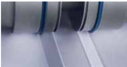
SCORING: The paper stock is undergoing a scoring process. The creases created enable easy folding and assembly of a packaging box for instance.
