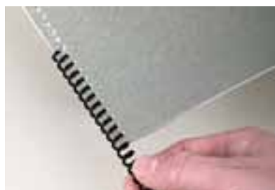
Wire-O bind is a series of parallel wire loops attached along a wire.
